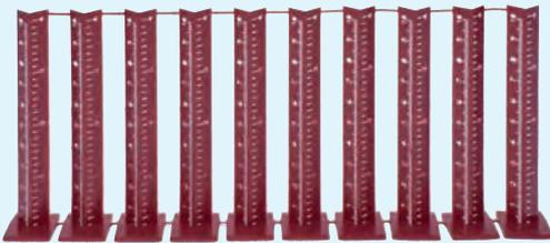
Simply cut the level pin with scissors to the desired height, using the moulded millimetre rule along the pin. broomstick the pin to the floor using the heavy-duty self adhesive base of the pin. Apply the concrete or screed until they are level with the top of the pin.
