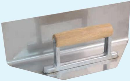
**stainless, blade thickness 1,2 mm, bevelled edges 45°, plinth height approx 10 cm, width 30 cm**
