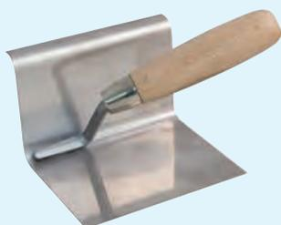
**stainless steel, blade thickness 1,2 mm, one side bevelled 90° with edge approx. 13 mm, plinth height approx. 8 cm, width 13 cm**
