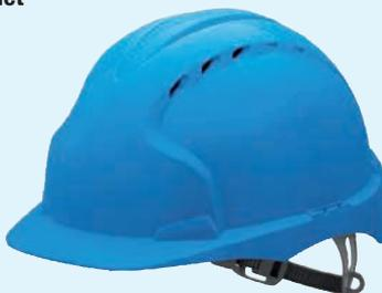
**with 6-point webbing interior, rotary knob to adapt to the head size, sweatband, rain gutter, ventilation, plug-in slots for hearing protection, made of polyethylene, weight approx. 340 g, color: blue**
