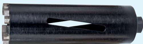
**Dry core drill for unreinforced concrete, mounting M16, segment height approx 10 mm, max work height 16 cm, outside diameter 57 mm, inside diameter 50 mm**
