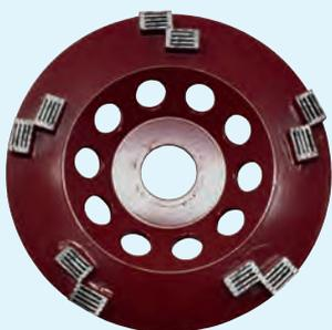
**for quick and easy removal of varnishes and paints, very aggressive, best design for the removal of paints and coatings, segment height 6 mm, mesh 16/20, soft bond, hole diameter 22,2 mm**
