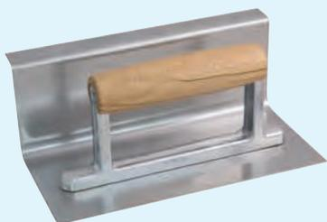
**stainless steel, blade thickness 1,2 mm, one side bevelled 90° with edge approx. 11,5 mm, plinth height approx. 7,5 cm, width 20 cm**
