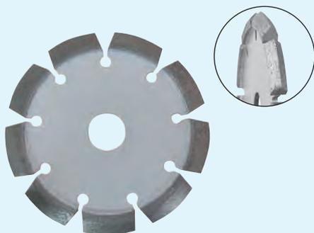
**to cut V-shaped joints into floors and walls, segment width 10 mm, segment height 12 mm**
