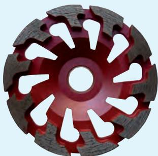
**for easy and fast removing of abrasive materials (cement screed/asphalt), very big suction holes for a fast suction. Delivery with a reduction ring from 25,0 to 22,2 mm, segment height 6,6 mm**
