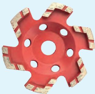
**suitable for plastic, paints, concrete, segment height 7 mm, mesh 30/40, medium bonding, hole diameter 22,2 mm**
