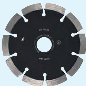
**suitable for abrasive materials e.g.. Cement screed, lime stone, fresh concrete, laser welded, segment height 10 mm, hole diameter 22,2 mm**
