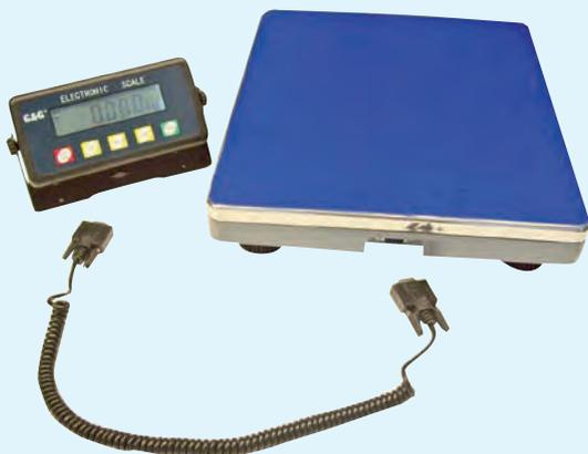
supporting platform 32 x 38 cm, weighing range up to 75 kg, up to 25 kg in 5 g steps from 25 kg in 10 g steps, TARA Function, automatic shutdown (idle) individually adjustable (deactivate, 15 min, 30 min, 45 min, 60 min), electric or battery powered (4x1,5V AA)
