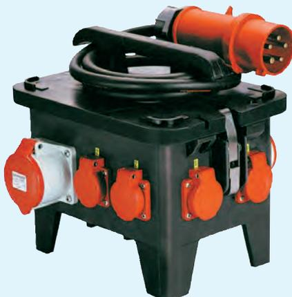
a closed housing substructure with a ground clearance of 77 mm prevents water ingress. Easy interchange of attachable sockets. Housing lid with quick-release, stainless-steel closure. Contact-protected according to BGV A2, also with the lid open. Additional security through installation of a screw or padlock
