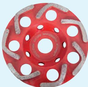
**suitable for plastic, paints, concrete, segment height 5mm, grit 30/40, medium/soft bonding, hole diameter 22,2 mm, Ø 150 mm 19 mm**
