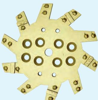
**Supreme quality, Ø 250 mm, for removing adhesive residues, floor coatings, paints, seals (EP, PUR, AC), plaster and fillers, screed and medium-hard fresh concrete up to grain 8, universal connection with 19 mm center hole and for M10, 20 segments 1/4 PCD and 5 support segments (MT-Design®) segment height 4 mm**
