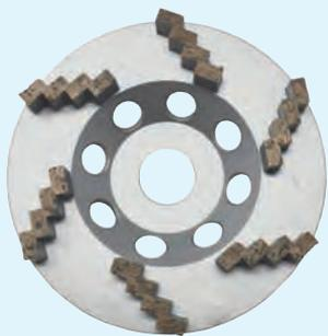
**for quick and easy removal of varnishes and paints, very aggressive, segment height 6 mm, mesh 16/20, soft bond, hole diameter 22,2 mm**
