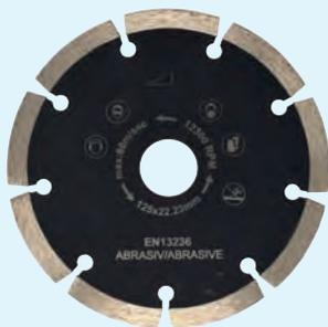
**suitable for abrasive materials e.g.. Cement screed, lime stone, fresh concrete, sintered, for wet and dry cutting, segment height 7mm, hole diameter 22,2 mm**
