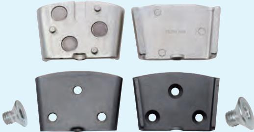
the shoe is assembled as usual and the diamond segments are placed on the adapter without screwing. The strong magnet holds the segment plate; the segment plate can be changed without tools.
