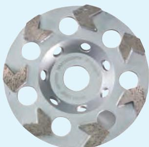
**for the removal of coatings on concrete, with several suction holes for optimal suction, segment height 5mm, mesh 30/40, medium bond, hole diameter 22,2 mm, Ø 150 mm 19 mm**
