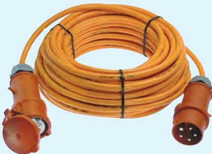
**CEE extension cable IP44, suitable for construction sites, workshops and industry. Polyurethane outer sheath with CEE plug and coupling with sealing cap, temperature resistant -40 to + 80 °C, with phase inverter plug**
