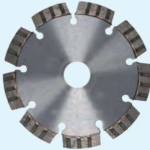
**turbo segments for fast cutting of reinforced concrete, concrete, concrete paver, laser welded, segment height 10mm, hole diameter 22,2 mm, Ø300-450 on request**
