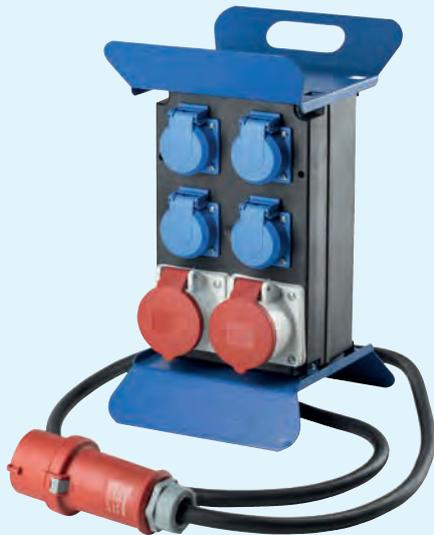
compact power distributor for construction site and outdoor use, IP44, housing made of special plastic highly resistant to breakage with a cable winder and carrying handle made of powder-coated metal
